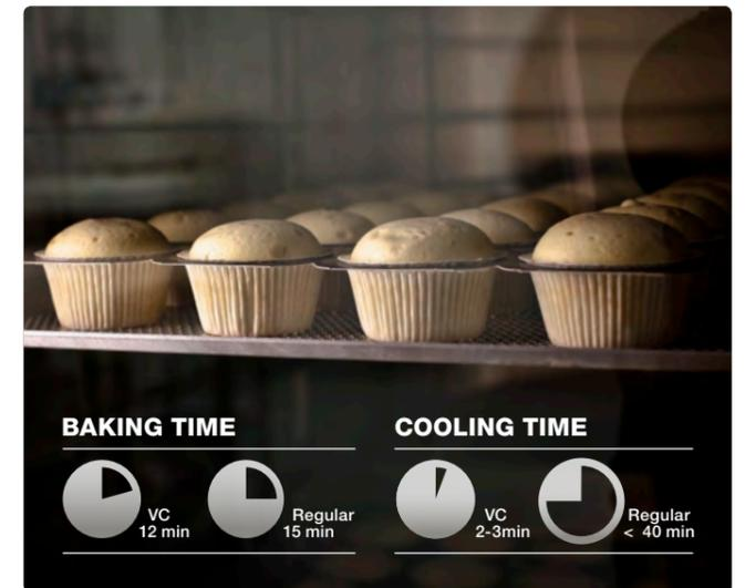
**2.** As the bread is allowed to finish baking during the vacuum cooling process, the total baking time is reduced with up to 30%. The actual cooling only takes a couple of minutes. Hence the baking and cooling time can be reduced to less than 15 minutes depending on products. This results in energy savings as well as less man hours needed. Also, you'll need less floor space due to fewer racks in the bakery.
